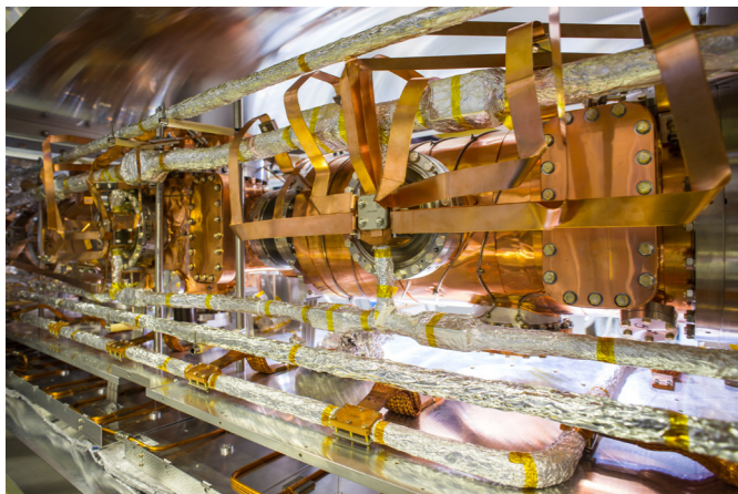
Copper strips distribute the cold in the cryogenic storage ring.
